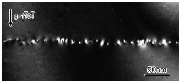
Fig. 3 A dark-field TEM image of the grain boundary obtained using the reflection g = (1\bar{1}0\bar{4}) . Small pair contrasts and relatively large contrasts can be seen along the grain boundary
